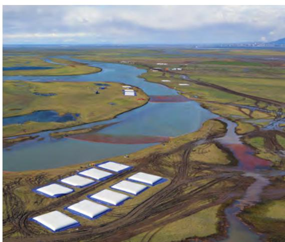
In June, seven teams of Transneft Siberia, JSC worked in the area of emergency recovery. The spilled diesel fuel was collected from the surface of the Ambarnaya River, its channels and oxbow lakes, using oil skimmers and containment booms. A total of 9,288 m<sup>3</sup> of petroleum products were collected from the water surface.
